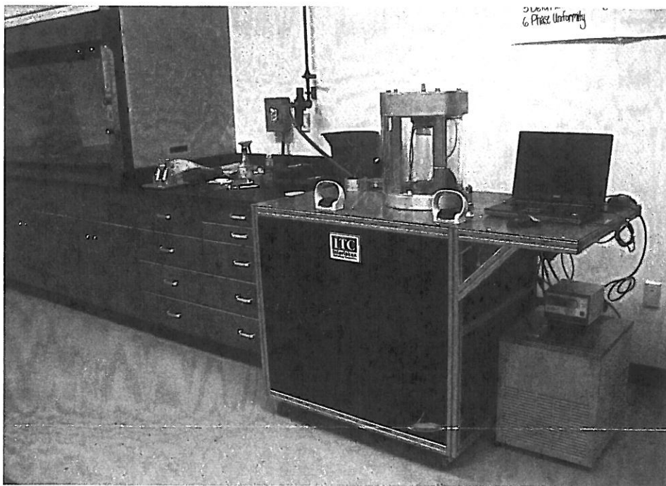
The asphalt mixture performance tester can subject a compacted asphalt mixture specimen to cyclic loading over a range of temperatures and frequencies.
