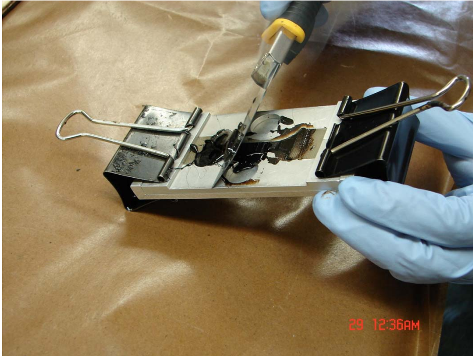
Step 13: Angle the mold downward and trim the excess sealants from the test mold.
