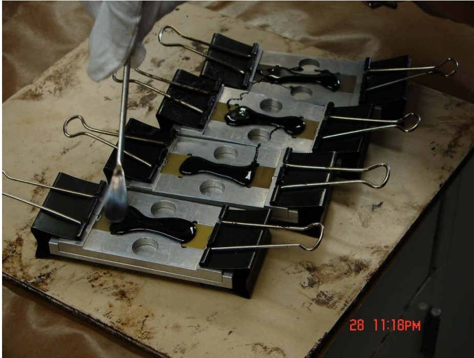
Step 11: Allow the test specimens to cool for 1hr at room temperature.
